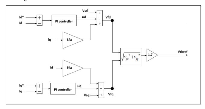
Fig 4.1: A block diagram of the DC-Bus reference voltage generation [30]
