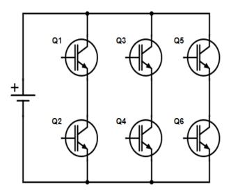
Fig. 3.5: A two-level inverter topology.
