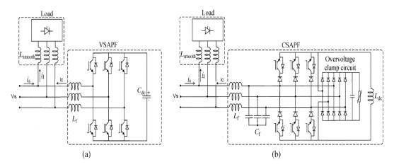
Fig. 2.6: Basic topology of : (a) VSAPF, (b) CSAPF.
