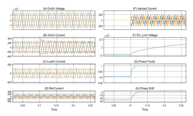
Fig. 6.15: Zoomed-in view of the waveforms of the SAPF showing its performance; (A) Grid's Voltages waveforms, (B) Grid's Current waveforms, (C) Load's Currents' waveforms,
