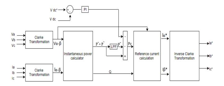
Fig. 3.1: Block diagram of P-Q theory for a reference current calculation.
