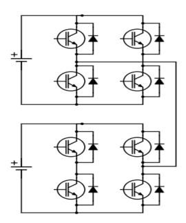
Fig. 3.8: A single phase of a five-nine level Cascaded Inverter.
