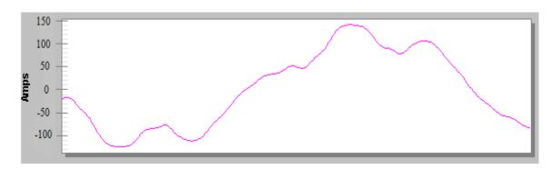
Fig. 6.32: Current waveform of selected feeder taken by data logger (DENT device).
