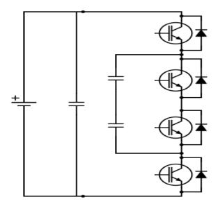
Fig. 3.7: A single leg of a Three-level Flying Capacitor Inverter.
