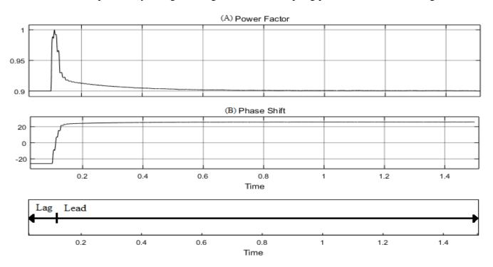
Fig. 6.22: Adaptive Power Factor from 0.9 lag to 0.9 lead.
