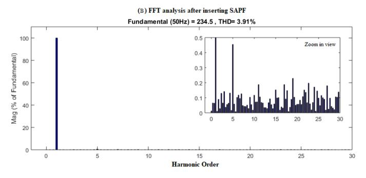
Fig. 6.17: FFT analysis of grid's current before and after inserting SAPF.
