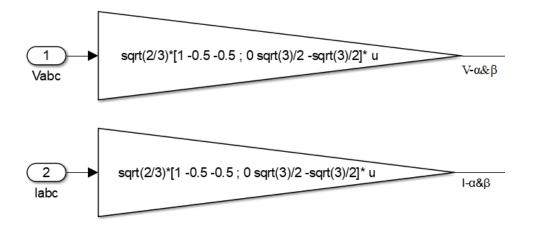
Fig. 6.4: α-β values calculation by Clarke transform
