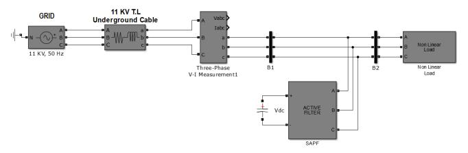
Fig. 6.1: The block diagram of a SAPF connected into a MV grid (11 KV).
