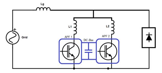
Fig. 2.10: Parallel SAPF block diagram
