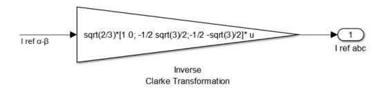
Fig. 6.8: Reference current calculation block diagram in a three-phase system.
