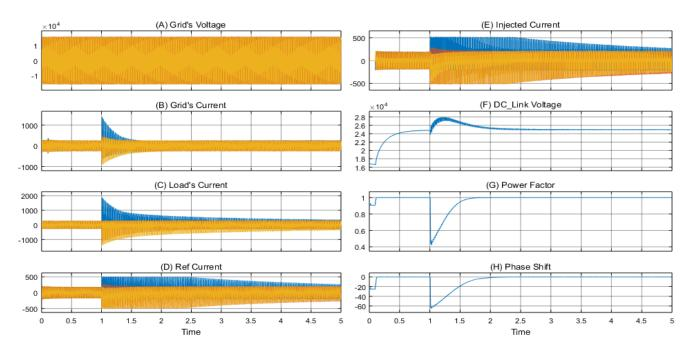
Fig. 6.28: The SAPF performance during energizing a distribution transformer (the inrush current)
