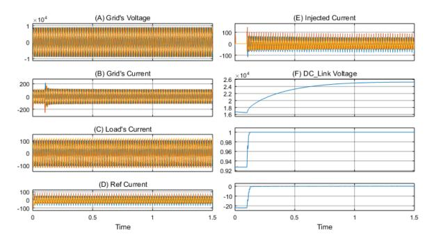
Fig. 6.33: The SAPF performance when implemented in the real case study
