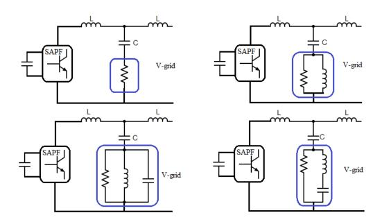
Fig. 2.9: Different damping circuits used with LCL filters.
