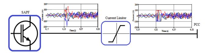
Fig. 5.2: A digital current limiter for overload protection of SAPF.
