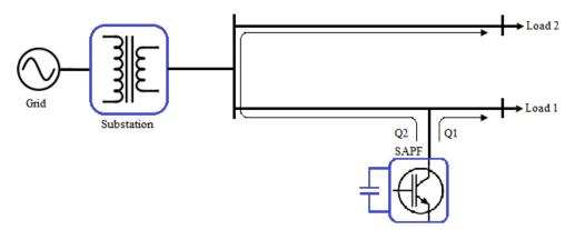
Fig. 5.1: SAPF provides reactive power to nearby load (Leading Case).
