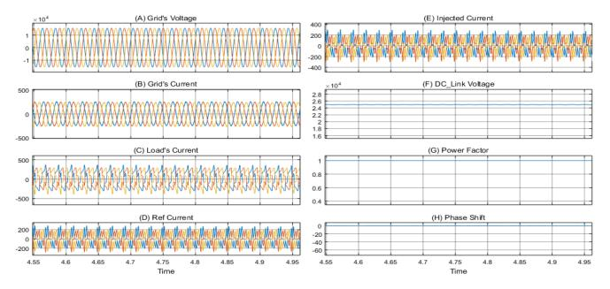
Fig. 6.29: A zoomed-in view of the SAPF waveforms during energizing a distribution transformer, with compensating harmonic distortion feature
