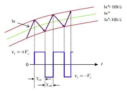
Fig. 2.7: Operating principle of Single Band Hysteresis Current Controller (SBHCC).
