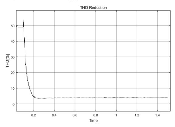
Fig. 6.16: The THD[%] is reduced when the SAPF was inserted across the nonlinear load at t=0.1s.
