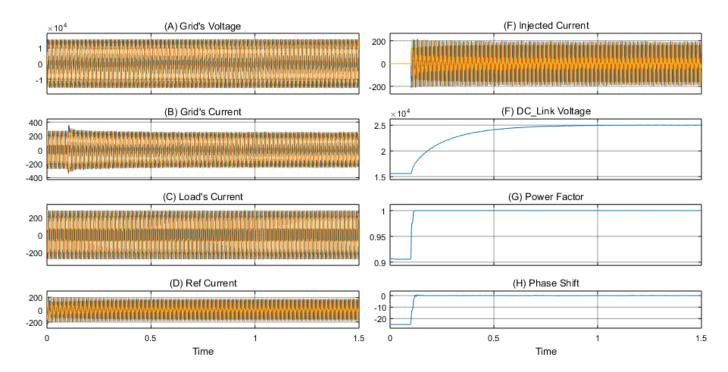
Fig. 6.18: The SAPF performance with Two-level inverter; (A) Grid's Voltages waveforms, (B) Grid's Current waveforms, (C) Load's Currents' waveforms, (D) Reference Currents' waveforms, (E) SAPF Injected Currents' waveforms, (F) DC-Link charging curve, (G) Combined Power Factor and (H) Phase Shift regulation curve
