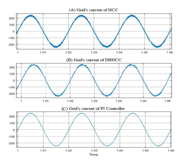
Fig. 6.21: Grid's current waveforms after inserting SAPF implementing; (A) HCC, (B) DBHCC, and (C) PI Controller.
