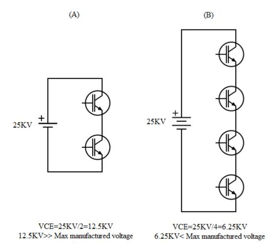
Fig. 6.20: DC-Link voltage distribution on bridge switches; (A) Two-level SAPF, (B) Multilevel SAPF.
