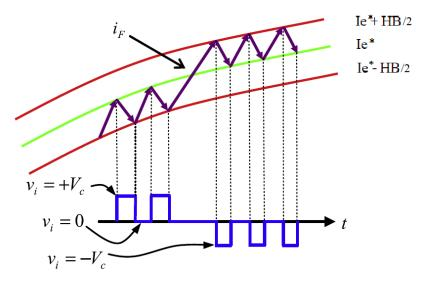
Fig. 2.8: Operating principle of Double Band Hysteresis Current Controller (DBHCC).
