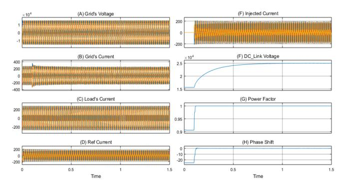
Fig. 6.14: Shunt-APF performance; (A) Grid's Voltages waveforms, (B) Grid's Current waveforms,
