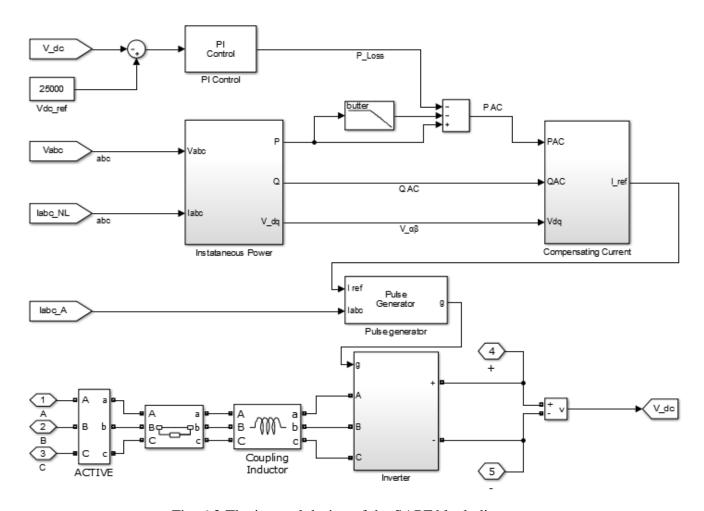
Fig. 6.3:The internal design of the SAPF block diagram.
