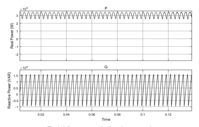
Fig. 6.11: Instantaneous real and reactive power results.
