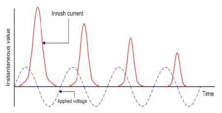
Fig. 5.4: Inrush current waveform.
