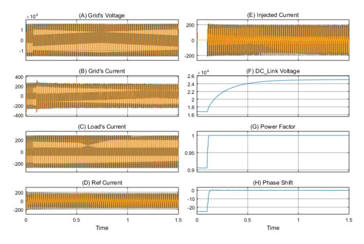
Fig. 6.19: SAPF performance with Multilevel inverter; (A) Grid's Voltages waveforms, (B) Grid's Current waveforms, (C) Load's Currents' waveforms, (D) Reference Currents' waveforms, (E) SAPF Injected Currents' waveforms, (F) DC-Link charging curve, (G) Combined Power Factor and (H) Phase Shift regulation curve
