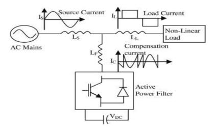
Fig. 2.5: Shunt Active power filters configuration.
