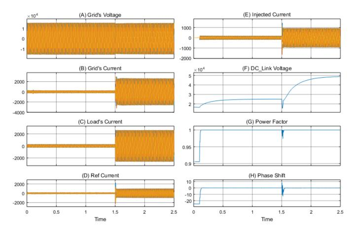
Fig. 6.25: Adaptive DC bus voltage behavior in fault conditions (Symmetrical Fault).
