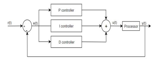
Fig. 3.4: A Block diagram of PID controller.
