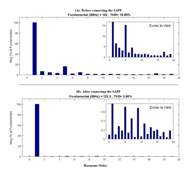
Fig. 6.35: FFT analysis of utility current, (A): before connecting the SAPF, (B): After connecting the SAPF.
