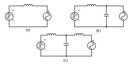
Fig. 2.2: Main circuit topologies of passive filters; (a) L, (b) LC and (c) LCL types [14].
