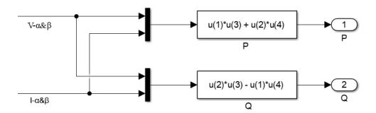
Fig. 6.5: Instantaneous power calculator block diagram
