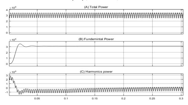
Fig. 6.12: Real power waveforms; (a) total consumed power, (b) power consumed by 50 Hz component, (c) Power consumed by other harmonics
