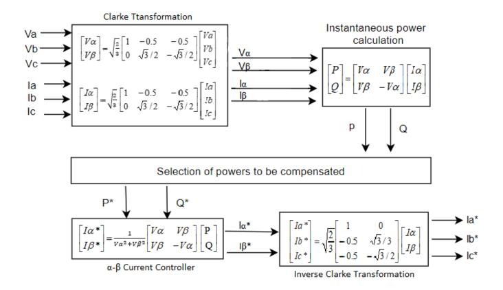
Fig. 3.2: Overall transfer matrices for reference signals generation.
