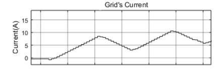
Fig. 6.10: Current ripple in a part of grid's current after inserting SAPF.
