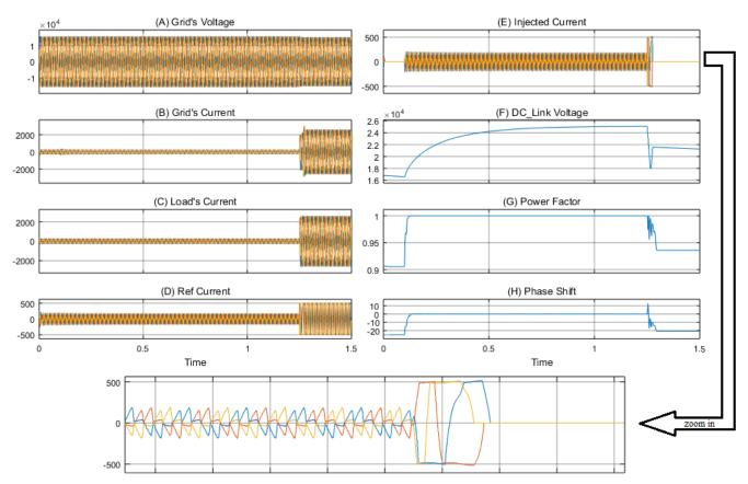
Fig. 6.27: Performance of SAPF protection during fault conditions
