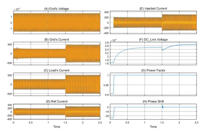
Fig. 6.24: DC bus voltage regulated by varying the connected load and increasing it up to twice the value of the connected load.
