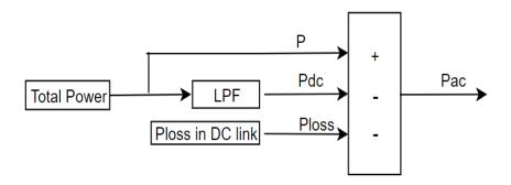
Fig. 6.6: Mechanism of selection the real power to be compensated.
