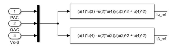
Fig.6.7: The model for reference current calculation in  $\alpha$ - $\beta$  system.
