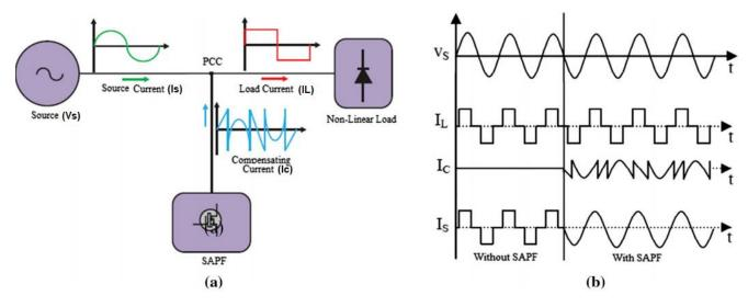
Fig. 2.1: General working concept of Active Power Filters; (a) block diagram of SAPF and (b) respective waveforms [9].
