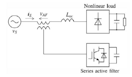
Fig. 2.4: A series Active Power Filter Configuration.
