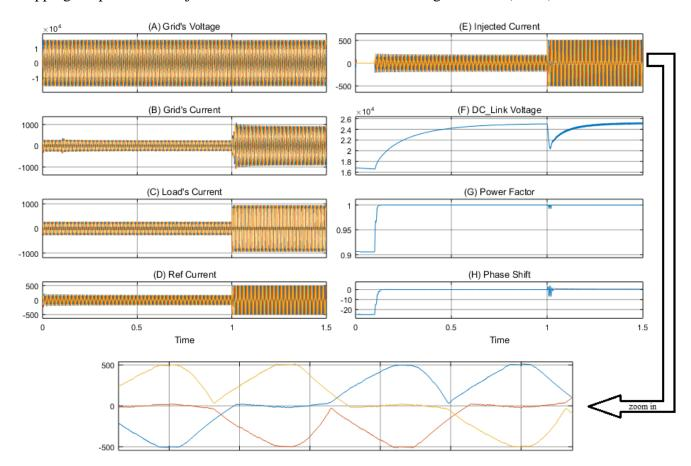
Fig. 6.26: The Current limiter performance in the SAPF protection from overload condition by clipping the peak current from exceeding the designed value (500A).
