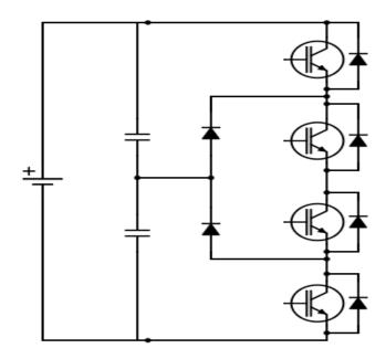
Fig. 3.6: A single leg of a three-level Diode Clamped inverter.
