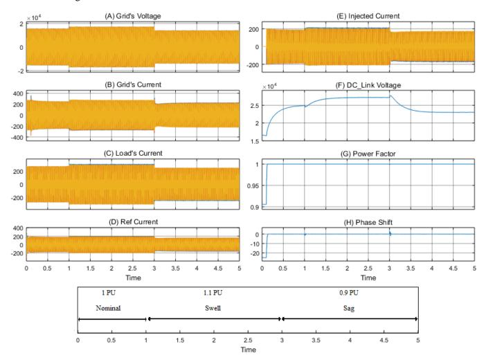
Fig. 6.23: Variation of the DC bus voltage when sag and swell events occur in the utility grid
