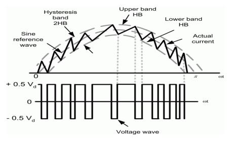
Fig. 3.3: Operating principle of Hysteresis Controller [17].
