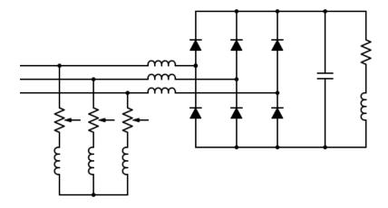
Fig. 6.2: Three phase AC/DC rectifier topology with adjustable Power Factor topology
