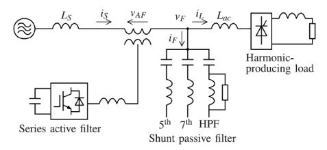
Fig. 2.3: The main configuration of hybrid filters.
