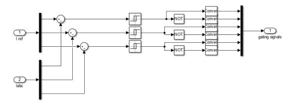
Fig. 6.9: Hysteresis Current Controller (HCC) simulation model
